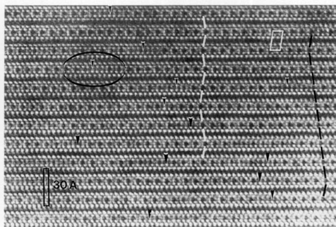
FIG. 17. HREM image of the 1222 compound, corresponding to the diffraction pattern of Fig. 16. The Pr configuration in the (Ca_{0.4}Pr_{0.6})O_8 plane is imaged as dark dots. The projected basic 1222 unit cell is outlined in black in the lower left corner, while the triclinic unit cell introduced by the in-plane ordering is outlined in the upper right corner. Antiphase lines have been indicated by vertical arrow heads.
